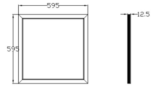
595mm x 595mm x 12.5mm mm 72W High CRI>83 Samsung SMD5630 leds
