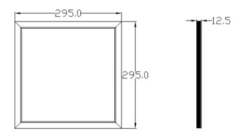
300mm (L) 300mm (W) 12.5mm (H) mm 36W High CRI>83 Samsung SMD5630 leds 2206lm 80% lumen maintenance at 40000 hours,
